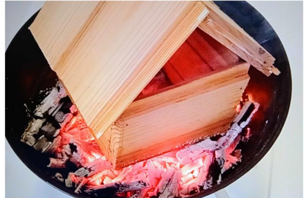
Fire-retardant treated wooden house on embers
