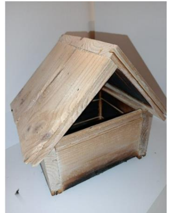
Fire-retardant-treated wooden house after burning
